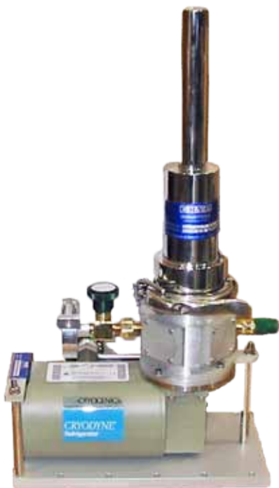
Custom Closed Cycle System for Narrow Gap Experiments
