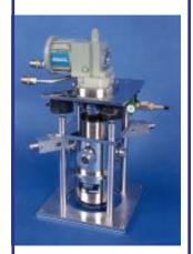
**CRYO** Industries closed cycle cryogenic WORKSTATIONS provide cooling without using liquid cryogens. Samples (chips) are mounted in vacuum into a chip holder (carrier). Designed for 'cold finger' sample mounting. Easy sample access through quick connect vacuum shroud. Large variety of standard optical shrouds and 'T' style mounts are available. Typical temperature operating range is from 10 to 325 K. Low vibration version for IR arrays or other vibration sensitive experiments is available.
