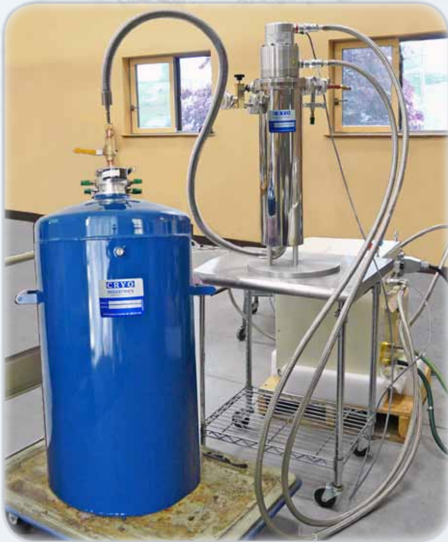
Cryocool-G2 Liquefier connected to portable storage dewar
