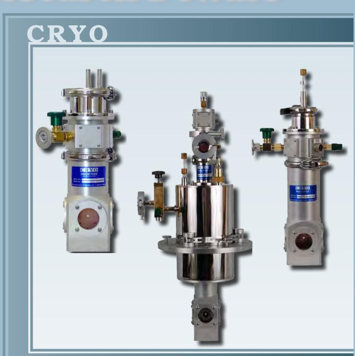
Cryo Industries Liquid Nitrogen Research Dewars are available in various styles that are sure to meet your experimental need. You select the style; exchange gas, flowing vapor or cold finger! In addition to our three styles of variable temperature liquid nitrogen research dewars, we also offer non-variable temperature dewar deigns. Following are the three styles of variable temperature liquid nitrogen dewars available.
