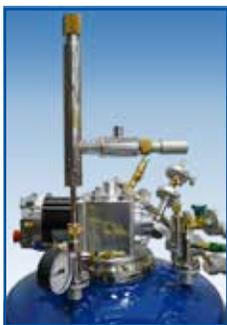
The integral liquid helium transfer line allows for simple, seamless transfers.
